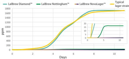
FI6. 4: H<sub>2</sub>S production during fermentation with LalBrew® Premium yeast strains for lager beer styles. A typical lager strain is shown for comparison purposes. Traditional lager strains (LalBrew Diamond™, typical lager strain) produce more H<sub>2</sub>S than ale strains (LalBrew Nottingham™). H<sub>2</sub>S levels are undetectable for fermentations with LalBrew NovaLager™. Standard all-malt 15°P pale wort pitched with 1.5 million cells/ml/°P and fermented at 12°C.
