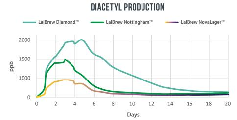
FIG. 7: The level of diacetyl produced by different yeast strains for lager styles.
