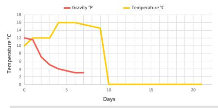
FIG. 5: A typical diacetyl rest is performed by increasing the temperature for several days at the end of active fermentation
